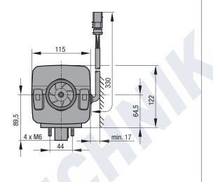
Minimum installation distance (clearance) for opening the cover
