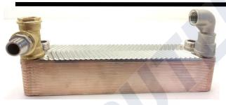
Attach Part A and Part B to your Heat exchanger as pictured above. Tip. Use plenty of PTFE on the heat exchanger threads to ensure a good tight connection and ensure open end of elbow points towards opposite port.
