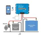
Isolated basically means that the input and output circuits don't share a common ground (negative), this is great for installations that don't share or cannot share a common negative for leisure and vehicle circuits, boats for example and vehicles which have sensitive equipment.
