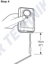
Turn the detector on its side so that the vents on the right hand side of the detector are pointing downwards (see diagram opposite). Hold the burning incense stick around 15cm (6 inches) below the detector, so that the smoke enters the vents on the side of the detector. An increase in the localised carbon monoxide
