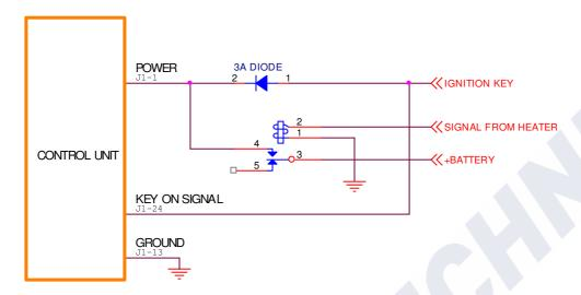
When the heater is activated (high voltage) the control unit is powered on and the key on signal is low.
