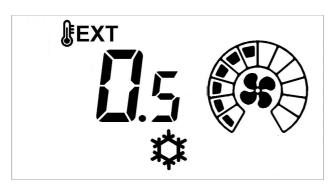
The symbol is on and the value displayed is not blinking to highlight that you are viewing the external temperature.
