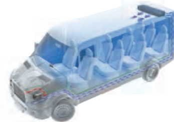
Evaporator under the roof
