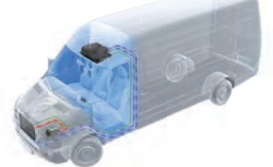
Evaporator integrated into the roof
