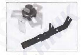
Removed sender unit viewed from above showing measurements to drill fuel pickup hole.
