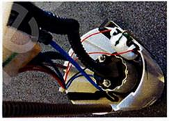
4. Route the blue fuel line inside the black guide within the sender unit to prevent unwanted interference.
