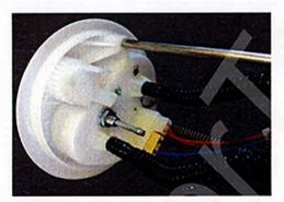
3. Using a 12mm spanner./Tighten sender pick-up pipe. Remove the nylon insert from the pick-up pipe. Then attach the 3.5mm rubber connection piece and ensure to butt the 230mm long blue fuel line to the fuel sender pickup and fasten using two 9mm clips.
