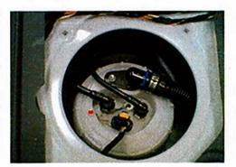
6. Ensure the sender is pushed all the way in when the lock ring, is tightened down. You may then re-connect the vehicle fuel and wiring connections.
