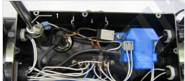
1 Socket spanner for series resistor
