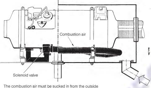
The combustion air must be sucked in from the outside (not from the passenger compartment or trunk) using the flexible tubing mounted to the heater without shortening or extending this tubing but leaving it unchanged.
