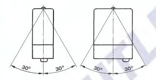
Fit the control unit so that it is protected from splash water (from both its own vehicle and preceding ones). Outside installation is thus not permissible. The unit is best arranged in the vehicle interior, with the plugs pointing downward.
