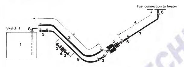
2. In the event of difficulties in fitting the riser pipe, the supply line can be tapped as shown in Sketch 2 in the case of diesel-engined vehicles and petrol-engined vehicles with a mechanical fuel pump.
