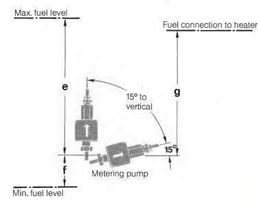
Supply pressure from tank to metering pump: e = max. 1000 mm
