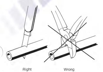
Connect up fuel pipes with a fuel tube. Fit the fuel pipe flush.
