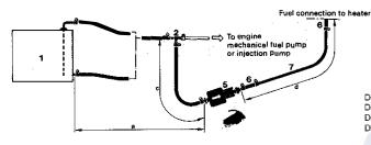
Dimension a = max. 5 m with diesel Dimension b = 50 mm Dimension c = max. 300 mm Dimension d= max~ 6 m with diesel
