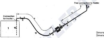
Dimension a = max. 5 m with diesel Dimension d = max. 6 m with diesel
