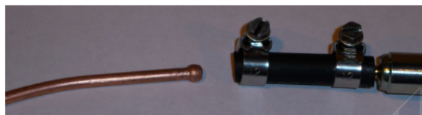
Flared end of copper pipe
