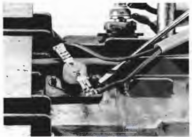
Fitting the safety thermal cutout switch
