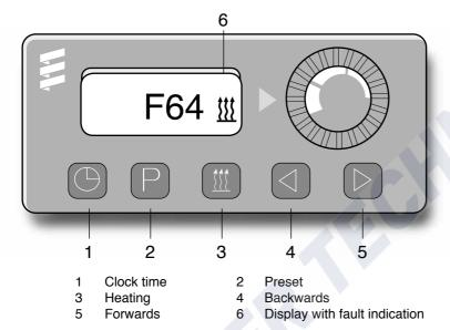
If the control unit detects a fault when the heater is switched on or while the heater is in operation, the timer module indicates this by means of an F and as a 2-figure number within 15 seconds.
